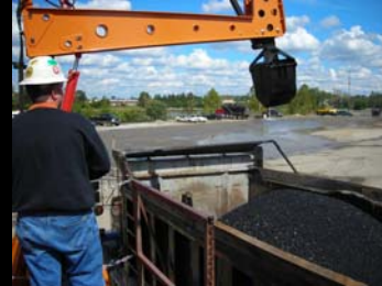
SAMPLER CAN BE POSITIONED OVER TRUCK
