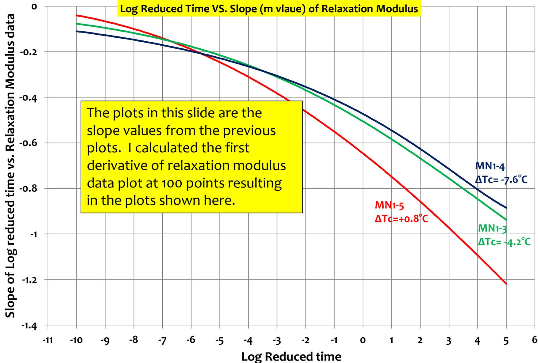
— slope MN1-5, 40 HR PAV RESIDUE — slope MN1-3 40 HR. PAV RESIDUE — slope MN1-4 40 HR. PAV RESIDUE
