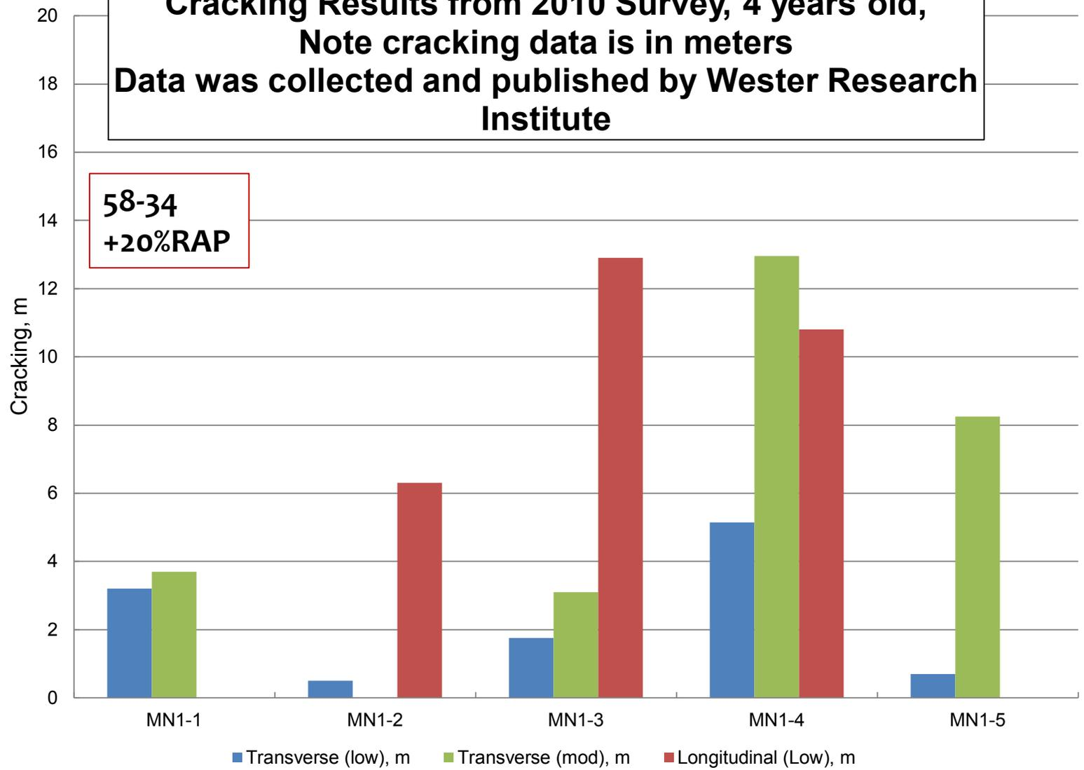
At 4 years there was not much total cracking in any test section , however sections MN1-3 and MN1-4 had the most cracking.
