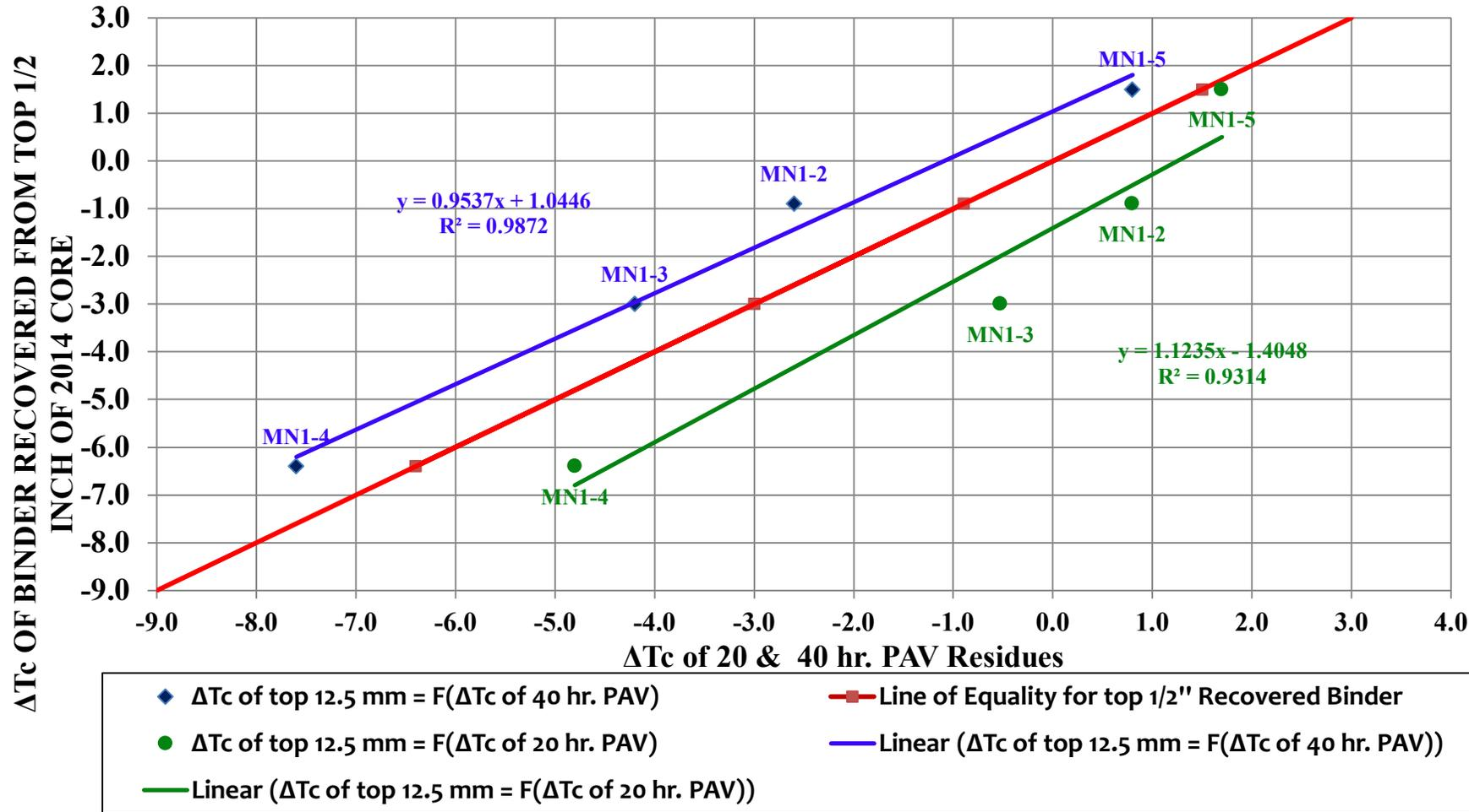
ΔTc of 20 HR. PAV UNDER PREDICTS THE ΔTc VALUE OF 8 YEAR FIELD CORE BINDER (TOP 1/2") TO A SLIGHTLY GREATER EXTENT THAN THE 40 HR. PAV OVERPREDICTS THE ΔTc VALUE
