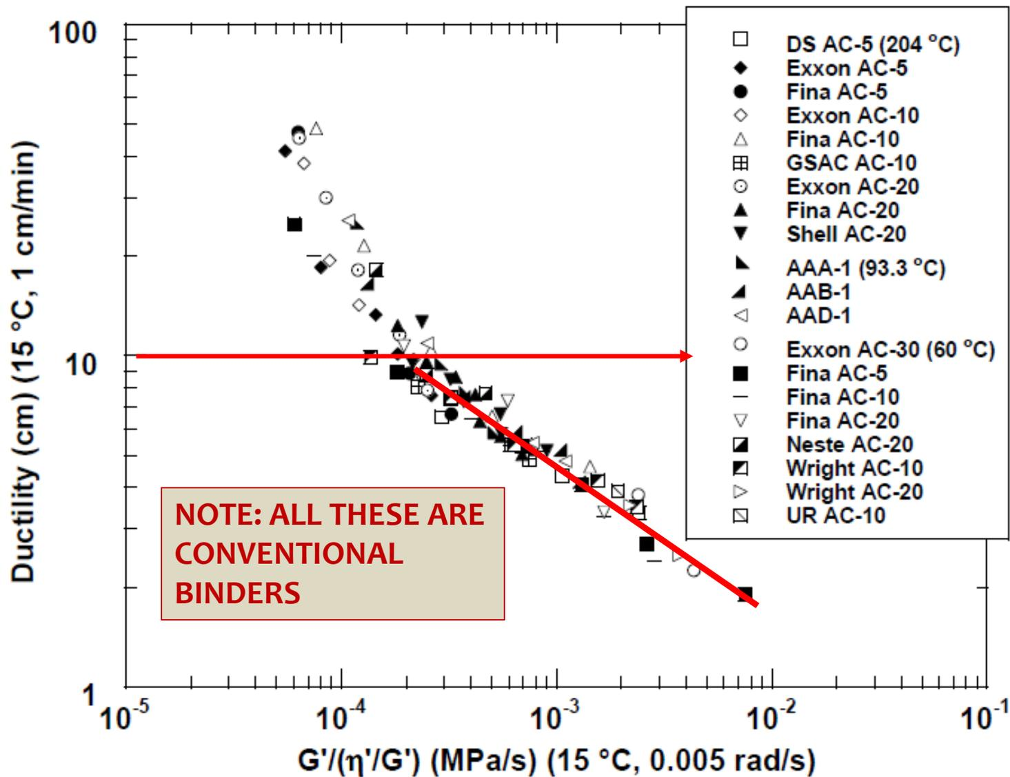
Figure 4-11. Ductility versus DSR Parameter  $G'/(η'/G')$ , All Ductilities.
