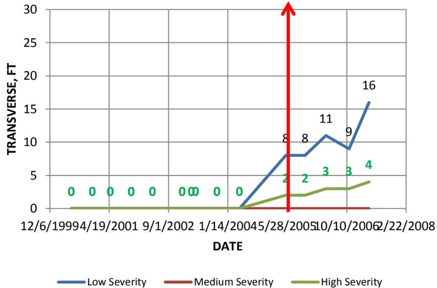
By year 5.5 some transverse cracking was appearing in all cells
