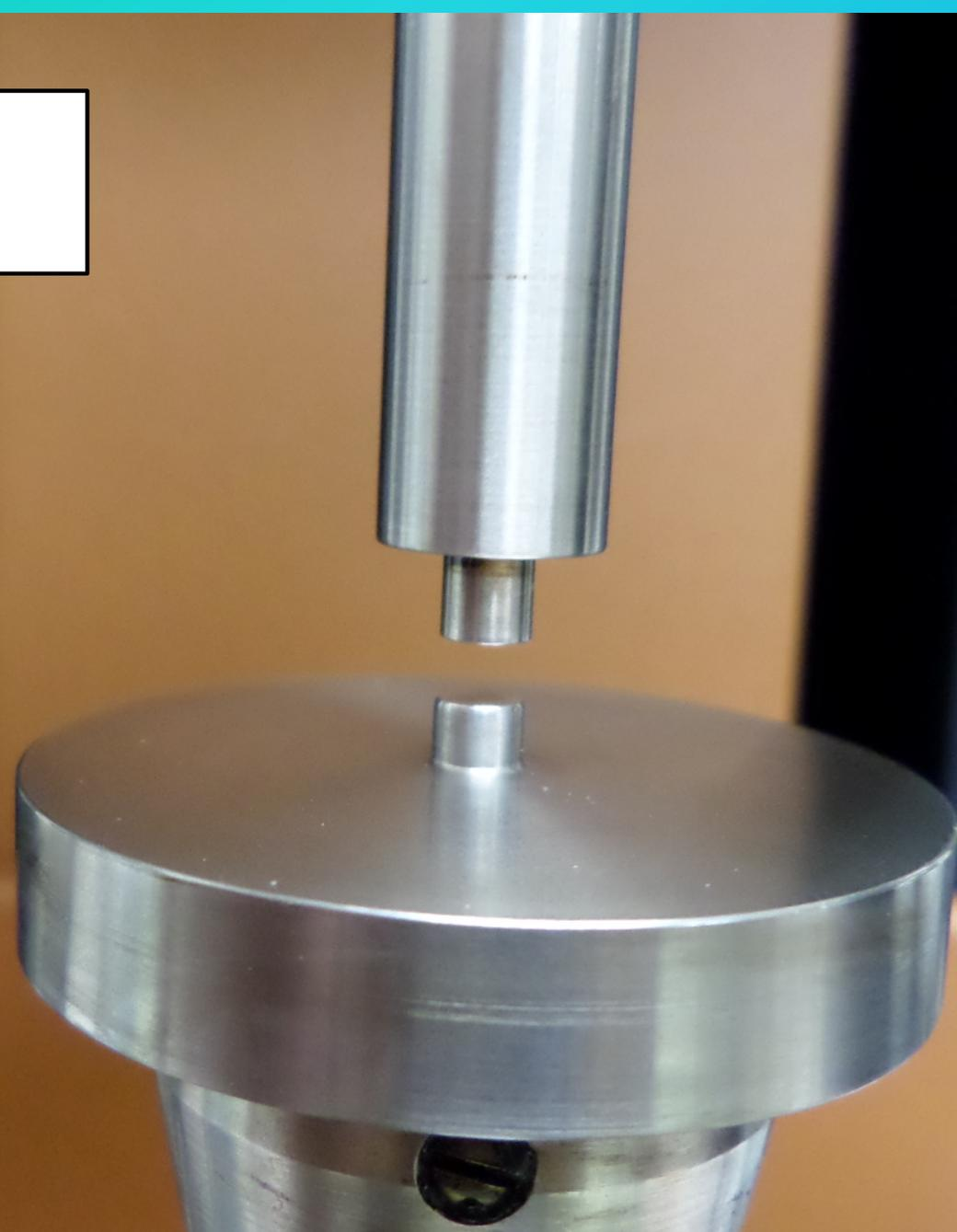
A picture showing a 4 mm diameter cylinder of metal to provide an image of the sample size of binder used in the test
