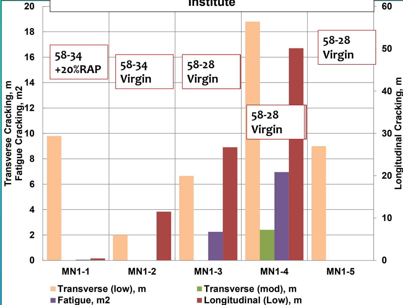
There was a substantial increase in cracking between years 4 and 5 especially for MN1-4
