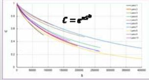
Path along which an asphalt mixture loses its structural integrity due to accumulation of damage (microcracks)
